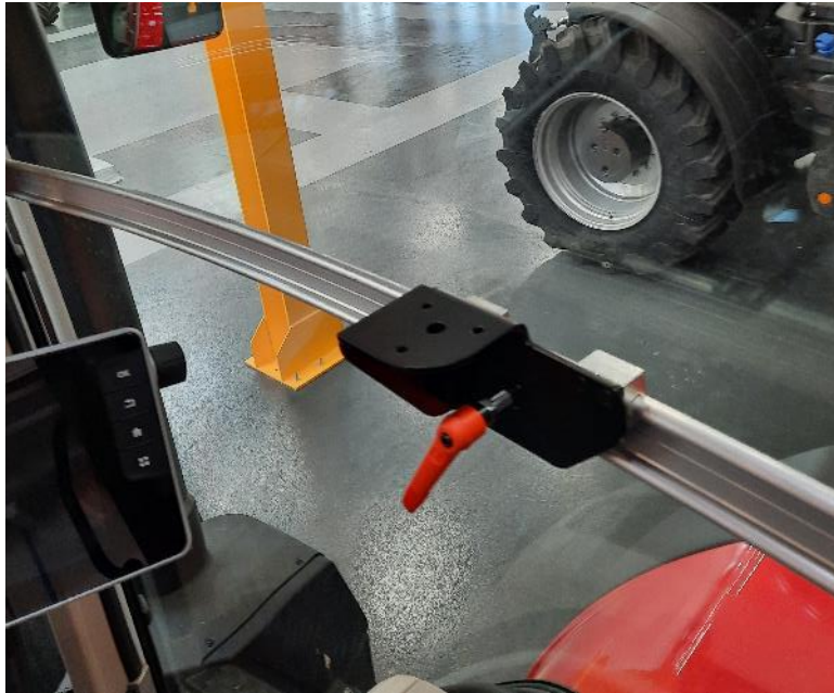
Screen support on the rail
