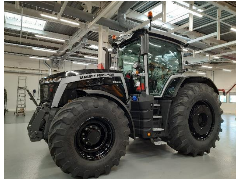
Black tractor : cab, hubs and rear wheels weights
