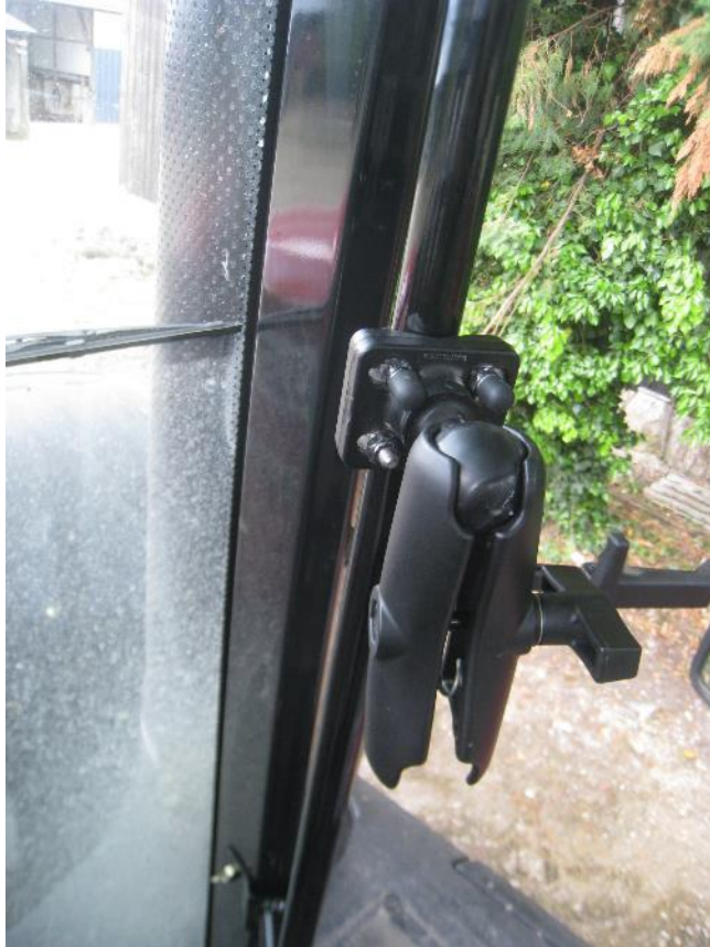
RAM screen support on A pillar bar
