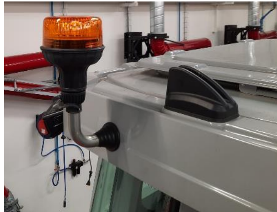
LED beacon replacing the standard one.
