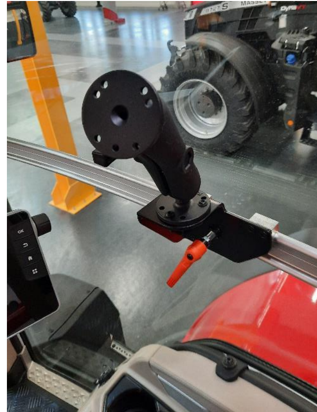
Screen support on the rail, including ram support
