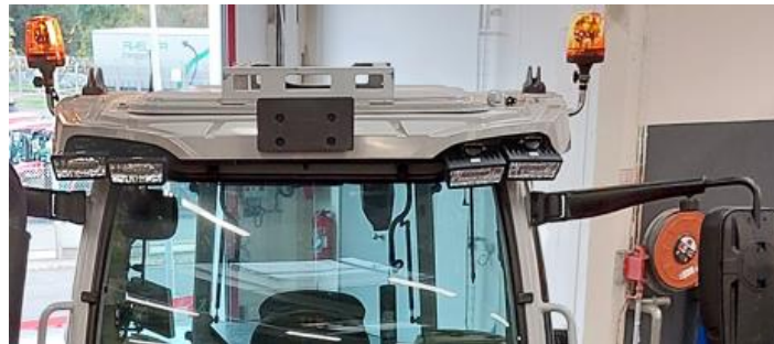
Plate support on roof
