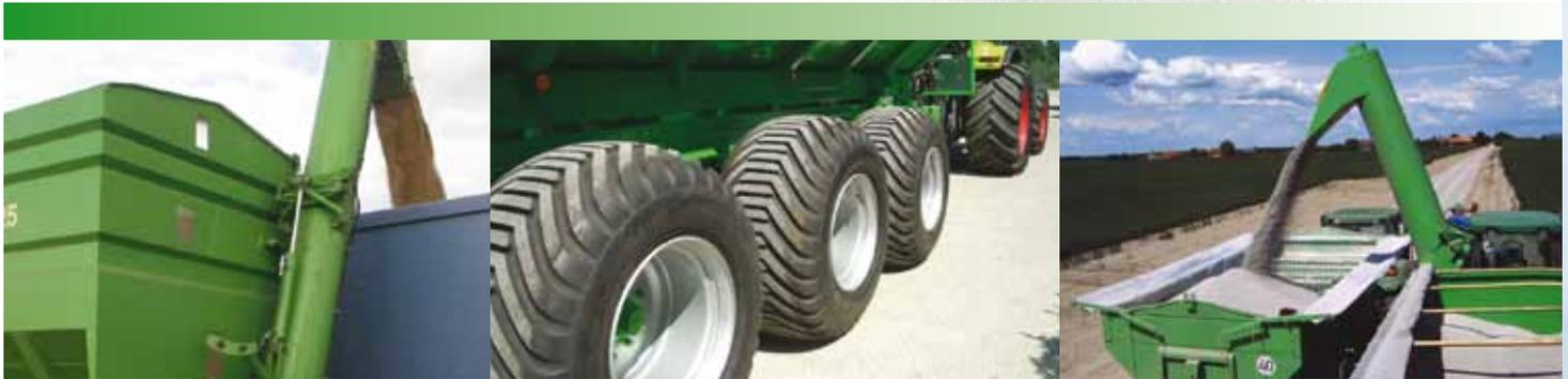
Large windows at the front of the hopper allow the operator full view of the bin loading, optional cameras in the bin and on the unloading auger help with this and the unloading operation.
