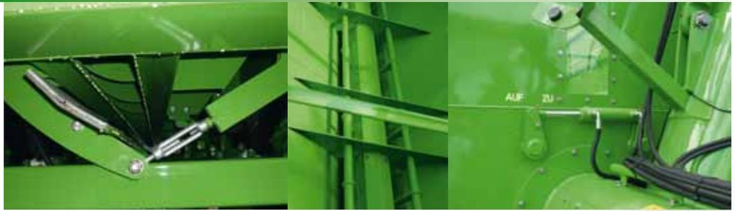
The complete emptying of remnants and easy hopper cleaning thanks to a manually operated trap door (over the whole length of the bin) allows for a quick turnaround when varieties are being changed. Two other large cleaning flaps are located at the bottom of the upright auger for a complete and Thorough clean.
